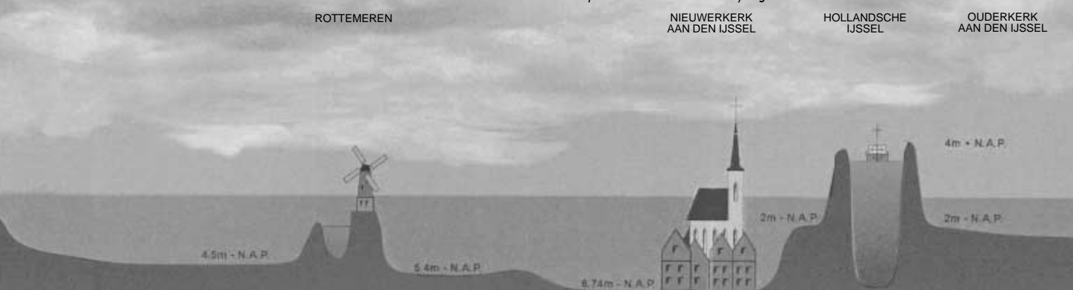
Partial cross-section of the Netherlands from the North-Sea to the lowest point at Nieuwerkerk a/d IJssel
